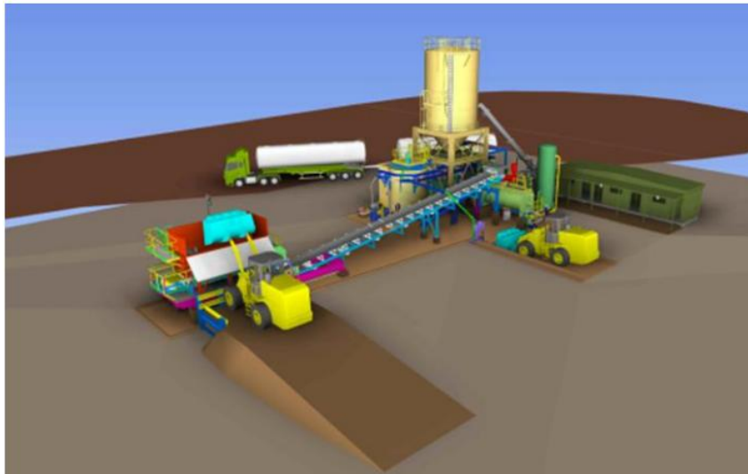
Figure 9: Never Never backfill plant isometric
