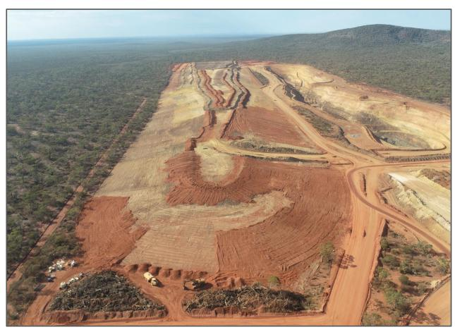
Figure 5: Topsoil spreading as part of ongoing rehab at Die Hardy pit (Marda)
