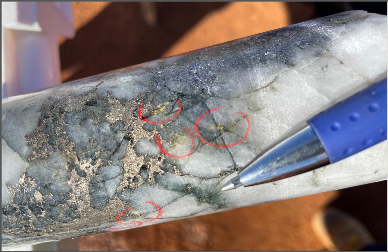
Figure 3: Finely disseminated visible gold ranging in size from 0.5-1.0mm in recent diamond core (PNDD009) within laminated quartz vein host rock at Penny North (4.5m intercept grading at 75.2g/t) with abundant massive sulphides (pyrrhotite+galena+pyrite) comprising up to 40% of the core volume associated with the gold mineralisation
