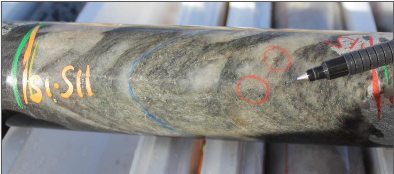
Figure 2: Finely disseminated visible gold in recent diamond core (PNDD004) within laminated quartz vein host rock at Penny Nth
