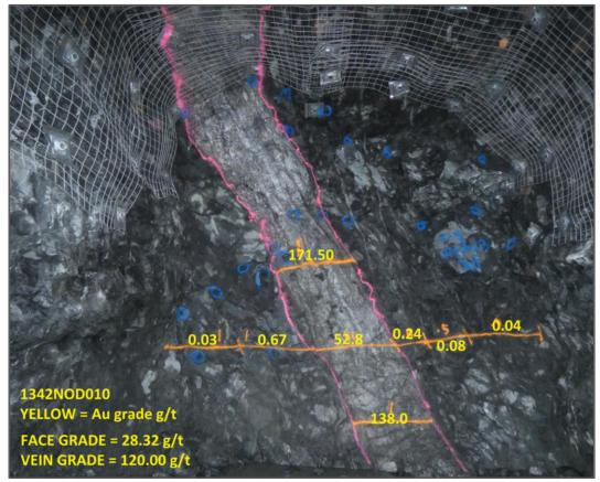
Figure 6: Face #10, 1342mRL north ore drive - face grade of 28.32g/t and vein grade of 120g/t
