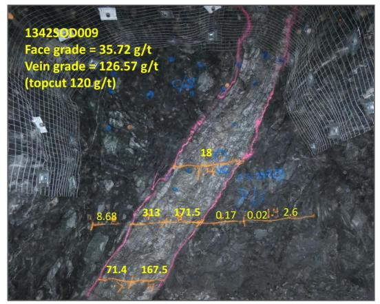
Figure 7: Face #9, 1342mRL south ore drive - face grade of 35.72g/t and vein grade of 126.5g/t
