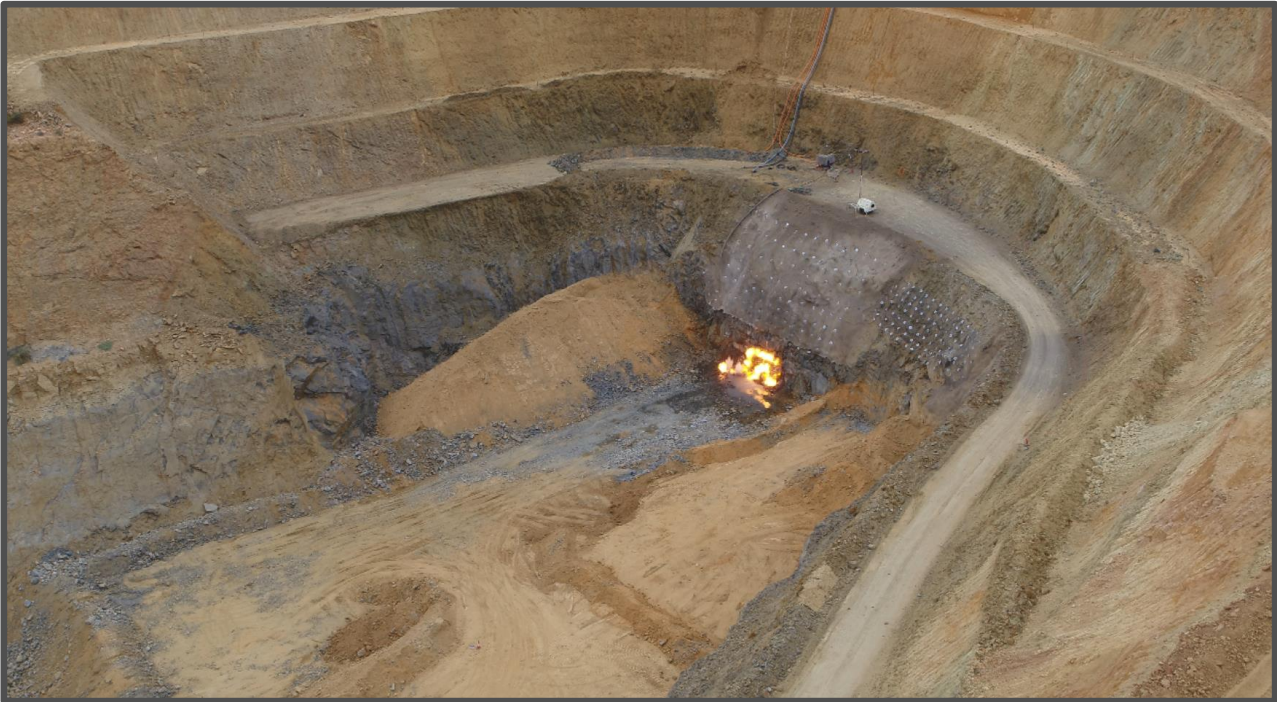
Figure 8: Penny underground portal firing
