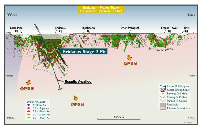
**Figure 7** – Exploration long section from Lone Pine/Eridanus through to Franks Tower/Jinx, highlighting the new hole (GXDD0104) and the untested potential that will become the focus of exploration drilling for the balance of FY2021
