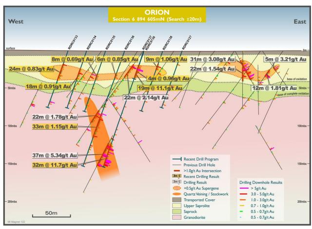
Figure 6: Orion cross section 6894605N - drilling results
