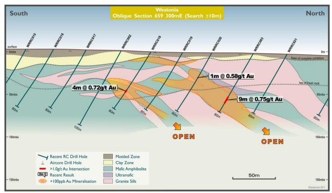
Figure 10 – Reconnaissance RC traverse located 1.5km west of the Greenfinch pit in an area previously believed to be entirely stoped by post mineralising granite sills
