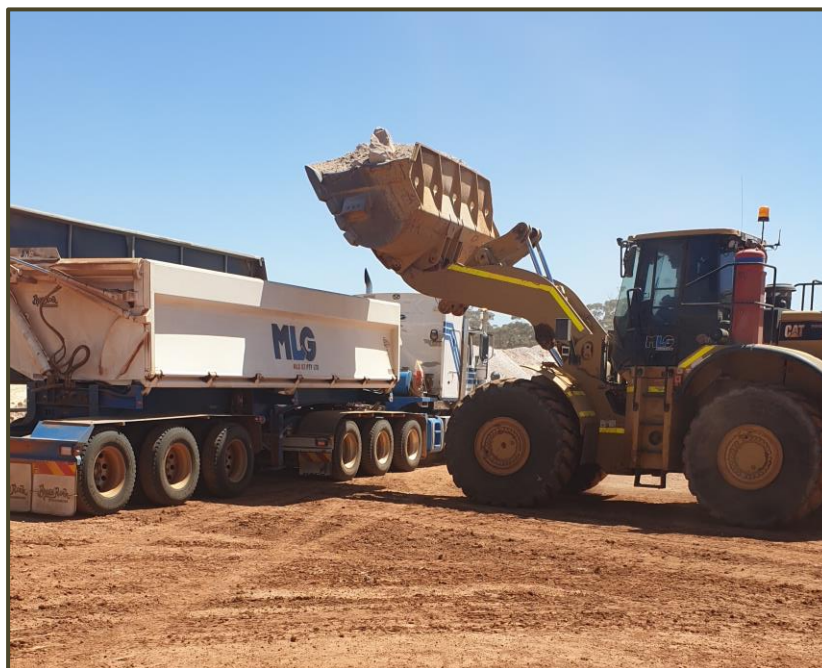
Figure 4: First ore haulage truck being loaded at Marda
