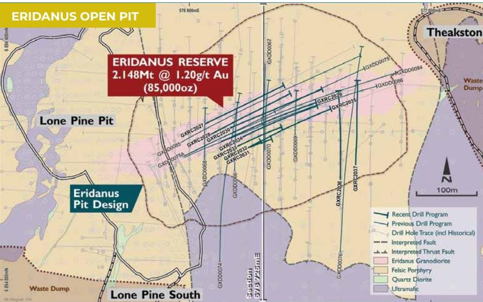
Detailed structural and vein density logging of the diamond core revealed a dominant subvertically dipping, north-westerly striking vein set within a broader stockwork vein array. The gold mineralisation is best developed within the competent east-west trending Eridanus Granodiorite but numerous lodes are seen to extend well beyond the granodiorite and are hosted by the surrounding Boogardie Basin felsic porphyry rocks.
