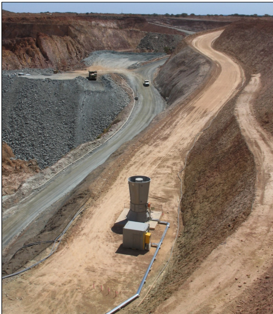
Figure 8: Vivien primary ventilation fan
