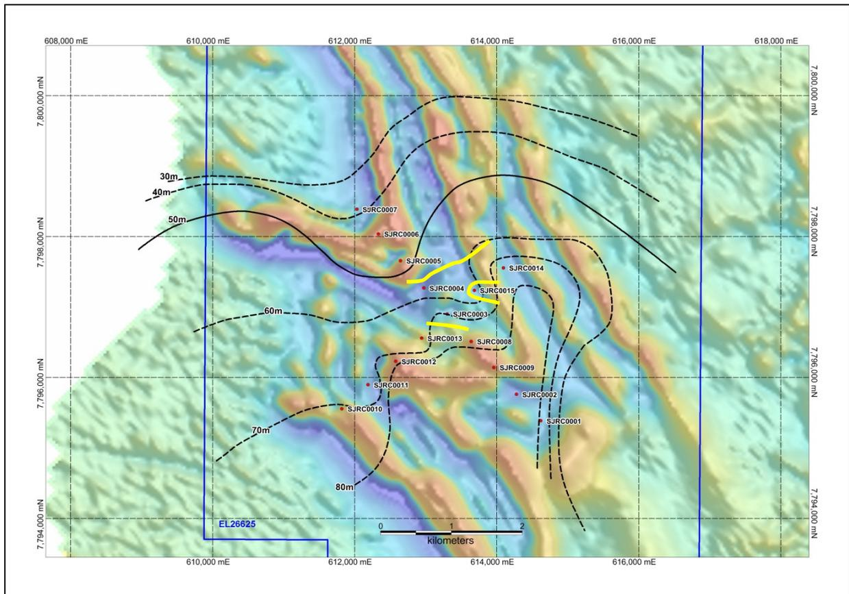
Figure 12: Suplejack (EL26625) showing Ramelius drill hole locations over an aeromagnetic image, highlighted the targeted folded Tanami Group stratigraphy. Black contours show the depth of unmineralised basalt cover. Yellow contours highlight an anomalous (plus 10ppb Au) interface trend between SJRC004 and 14 (over 1km), with results awaited from SJRC003.
