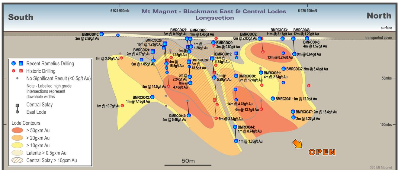
Figure 10: Blackmans East Lode longitudinal section highlighting the untested northerly plunge projection
