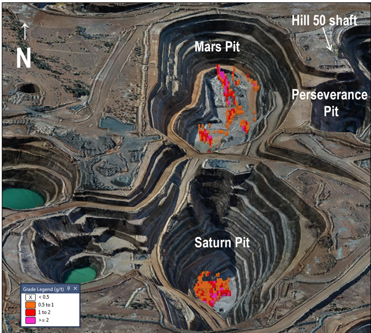
**Figure 3: Relative Positions of Saturn, Mars & Perseverance Pits in relation to the historic Hill 50 shaft**
