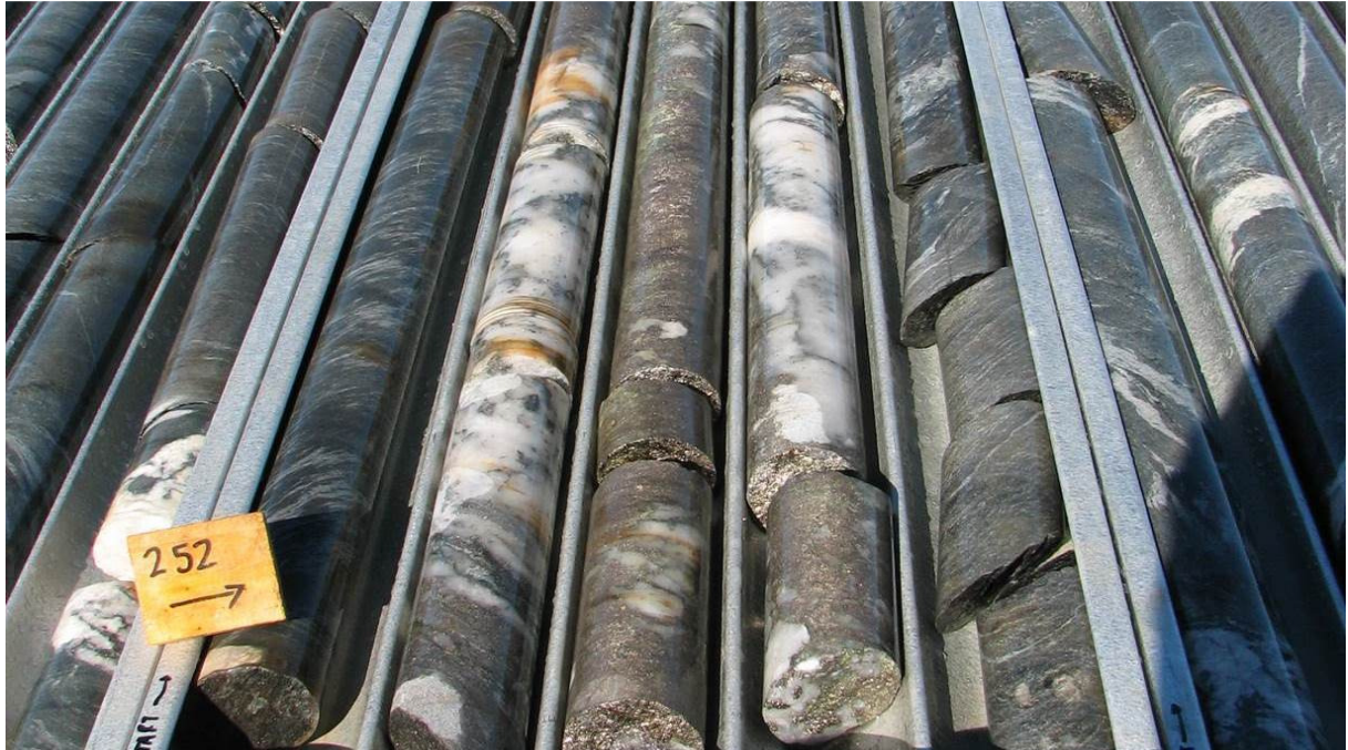
Photograph 1: Existing high grade Vivien drill core from hole VVDD176 (2.5m @ 78 g/t Au - true width 1.7m)
