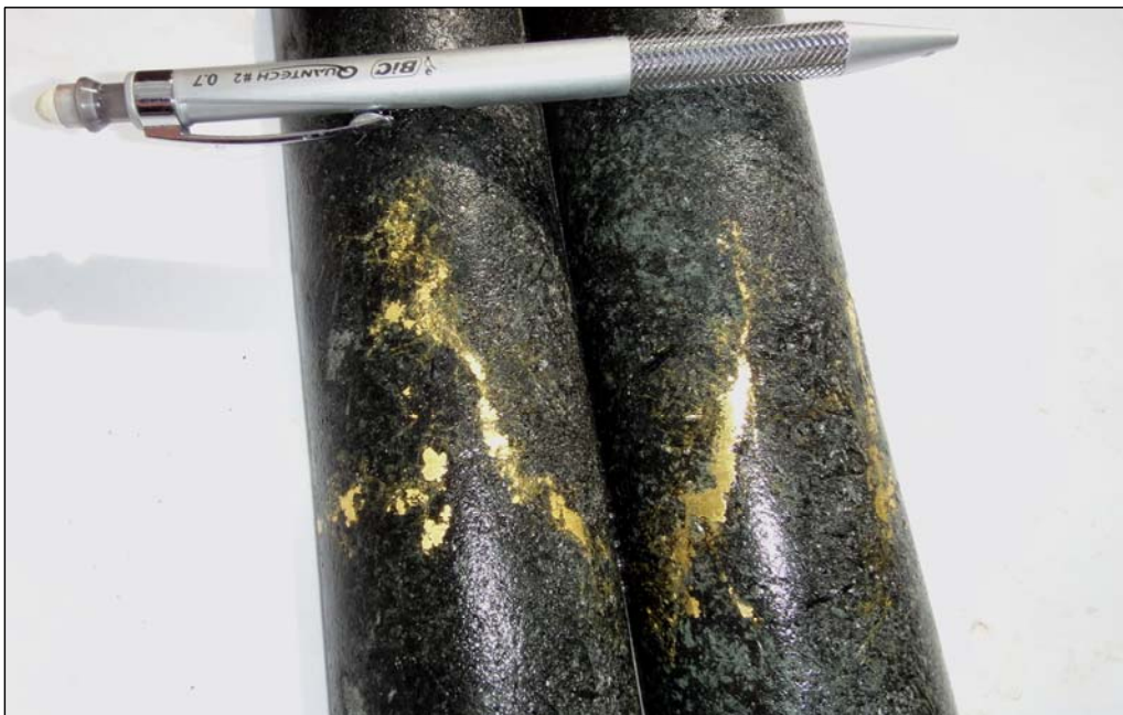
Figure 1. Visible gold in diamond hole WDUD0246 at the 100mRL (240m below surface)
