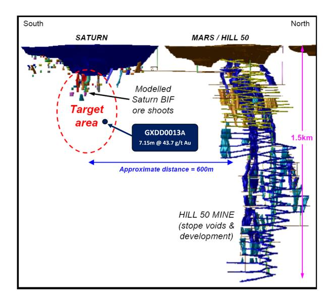
Figure 3: Cross section through Saturn at 80075mN showing the high grade intersection in GXDD0013A (312.45 g x m) relative to the proposed A\$1150 Galaxy pit shell (thick black line) and the existing resource block model.
