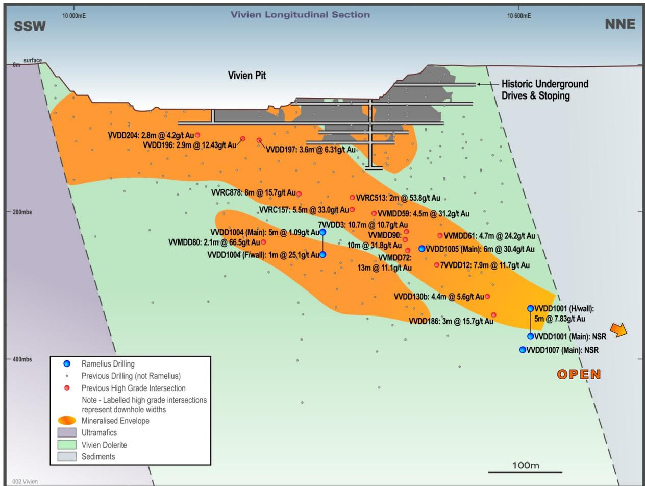
Figure 2: Longitudinal section – Vivien gold project
