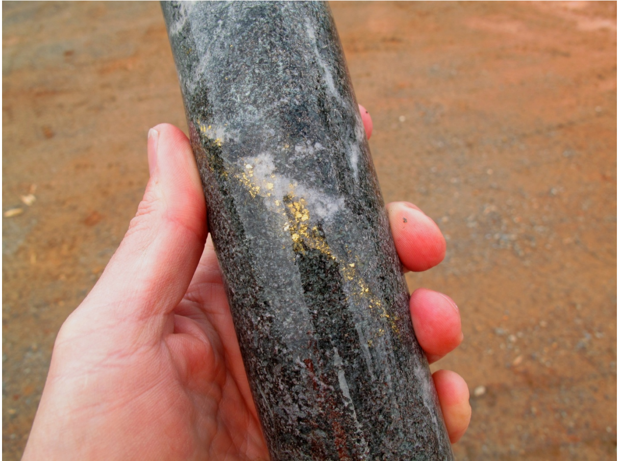
Photograph 1: Visible gold in WDUD0167 at 142m – assay results pending.
