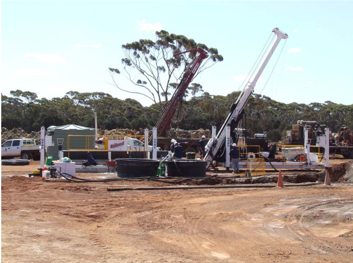
Figure 2: Diamond (foreground) and RC drilling rigs at Wattle Dam in September
